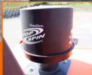
Centrifugal pre-cleaner Top Spin™ Donaldson® series
