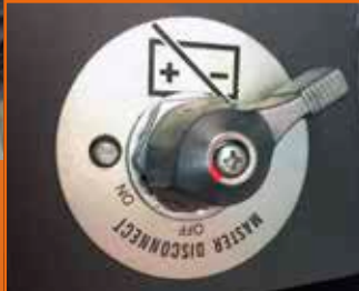
Battery cut-off switch
