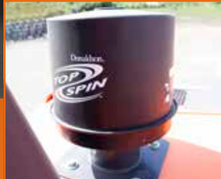
Centrifugal pre-cleaner Top Spin™ Donaldson® series
