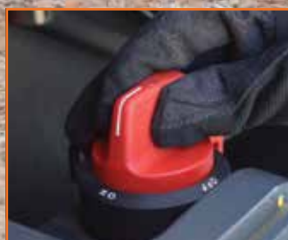
Battery cut-off switch
