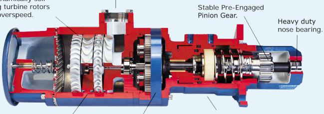
Large open air passages resist erosion and tolerate contaminants that could destroy other starters.
