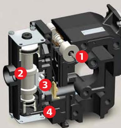
**1) SimulShift™ Valve:** Avoids stall-out - Provides faster pump trip-over with more flow – **2) "Unbalanced" Major Air Valve:** eliminates pump stall-out, even under low air inlet pressures – **3) "D" Valve** for optimum energy efficiency while avoiding costly air "blow-by" - Ceramic construction for long service life – **4) Quick Dump™ Checks,** eliminates pump ice-up by diverting cold, wet exhaust air away from the major air valve.
